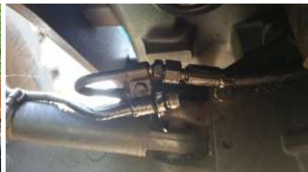
Image 28: Broken steering hose, Ambae, April 2016
