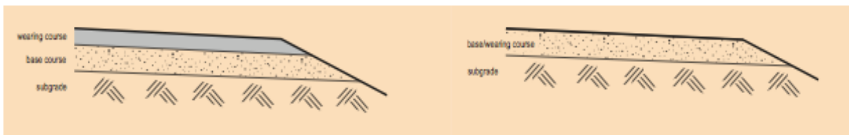
Figure 9 Pavement layer options
